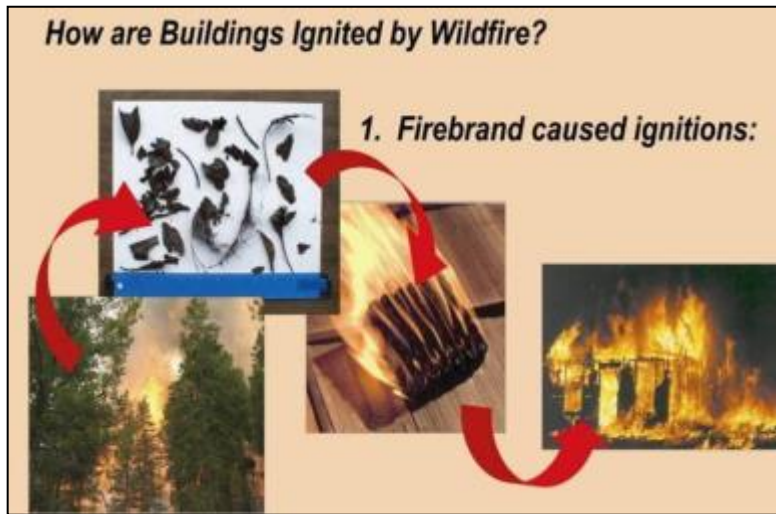
Figure 7. Firebrand caused ignitions: burning embers are carried ahead of the fire front and alight on vulnerable building surfaces.
