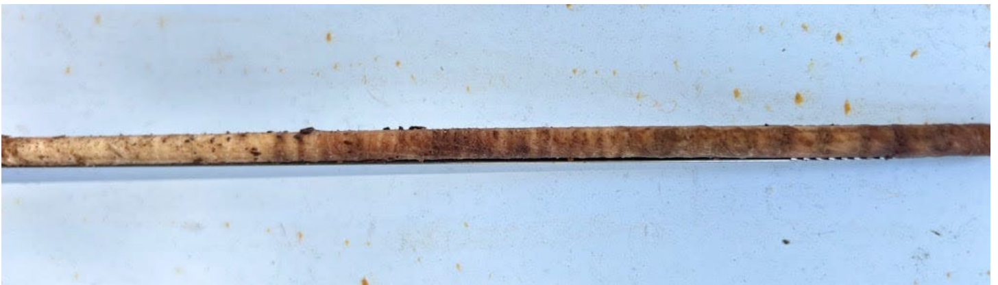
Fig.16 – Spongy texture observed with indication of decay throughout core sample.
