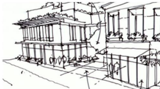
Ground floor setbacks incorporating patios, cafés and displays help animate the streets and public spaces.
