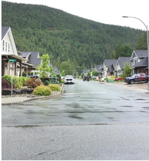
Figure 9. Example of wide residential roads and highly visible street addresses, facilitating effective emergency response.
